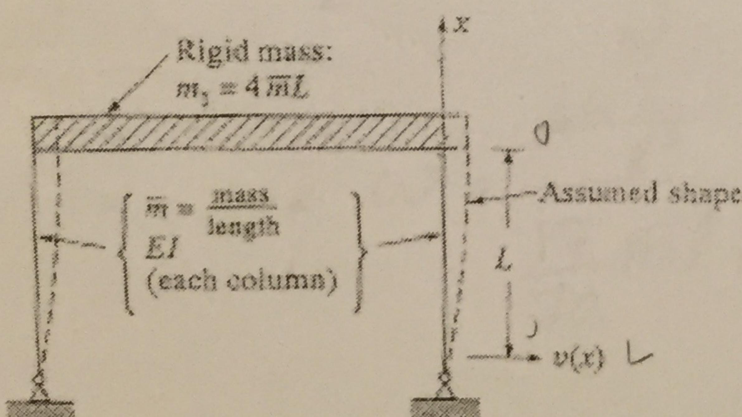
3. The shear building of Fig. 8 has its entire mass lumped in the rigid girders. For the given mass and stiffness properties, and assuming a linear initial shape (as shown), evaluate the period of vibration by: Rayleigh's method.
