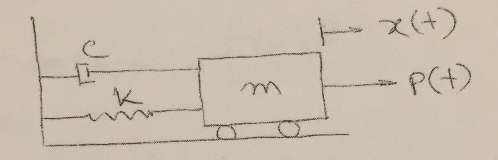
A control console containing delicate instrumentation is to be located on the floor of a test laboratory where it has been determined that the floor slab is vibrating vertically with an amplitude of 0.03 in at 20 Hz. If the weight of the console is 800 lb, determine the stiffness of the vibration isolation system required to reduce the vertical-motion amplitude of the console to 0.005 in.
