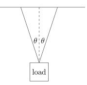
The (scalar) tensions  $T^{\text{left}}$  and  $T^{\text{right}}$  in the two cables are independently controllable, from 0 up to a given maximum tension  $T^{\text{max}}$ . The total force on the load is
