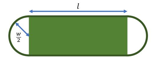
The basic idea is that the elastic cord loop goes through the top and bottom edge of the filter and forms two half-circles at its opposing ends. The filter is of width w and length l and must have a minimum area of  $300cm^2$  according to the standards. Moreover, they impose the following upper and lower bounds on the aspect ratio,
