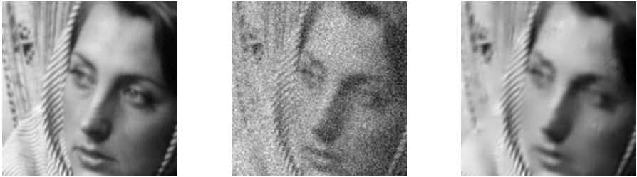
Fig. 5. From left to right: original image, noisy image with zero-mean white gaussian noise of \|\mathbf{n}\|_2 = 20 , the cleaned image via sparse representation described
