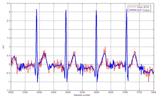
Figure 2. EKF output for ECG signals with erased
