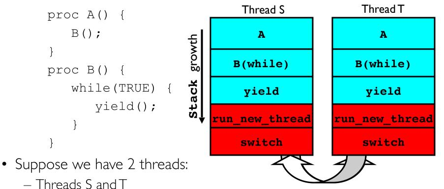
Thread S's switch returns to Thread T's (and vice versa)
