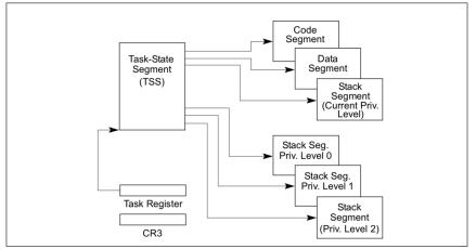
Figure 7-1. Structure of a Task
