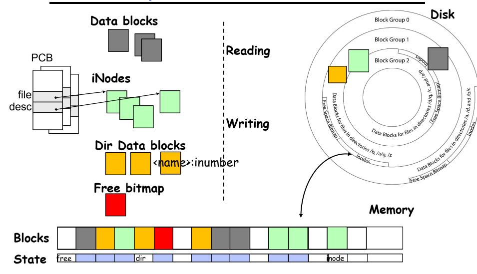
• From inode, traverse index structure to find data block; load data block; copy all or part to read data buffer
