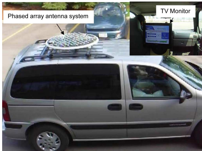
Fig. 11. The phased array antenna system mounted on a test vehicle.
