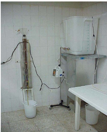
Figure 3.1. Experimental Set-up of HAIS and UASB reactors: (1) Influent synthetic substrate; (2) Peristaltic and Infusion pumps; (3) Sampling port; (4) Biogas collection system; and (5) Effluent. (a) HAIS-PU; (b) HAIS-PE; and (c) UASB;
