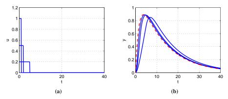
**Figure 5.6:** Pulse response and impulse response. The figure on the left shows pulses of width 5, 2 and 1, each with total area equal to 1. The corresponding pulse responses for a linear system with eigenvalues  $\lambda = \{-0.08, -0.62\}$  are shown on the right as solid lines. The dashed line is the true impulse response, which is well-approximated by a pulse of duration 1.
