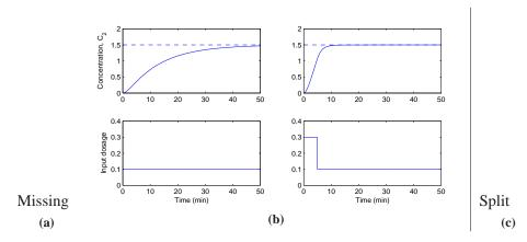
**Figure 5.10:** Response of a compartment model to a constant drug infusion. A simple diagram of the system is shown in (a). The step response (b) shows the rate of concentration buildup in compartment 2. In (c) a pulse of initial concentration is used to speed up the response.
