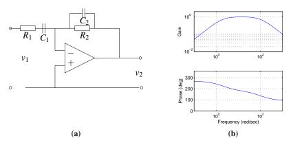
**Figure 5.12:** Active band pass filter. The circuit diagram shows an op amp with two *RC* filters arranged to provide a band pass filter. The plot on the right shows the gain and phase of the filter as a function of frequency.
