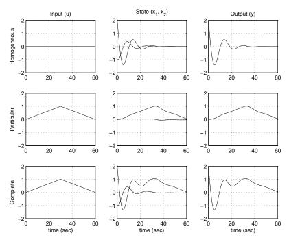
**Figure 5.1:** Superposition of homogeneous and particular solutions. The first row shows the input, state and output corresponding to the initial condition response. The second row shows the same variables corresponding to zero initial condition, but nonzero input. The third row is the complete solution, which is the sum of the two individual solutions.
