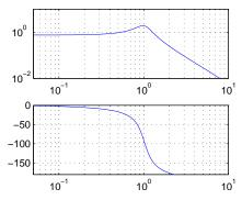
**Figure 5.11:** Frequency response, showing gain and phase. The gain is given by the ratio of the output amplitude to the input amplitude,  $M = A_y/A_u$ . The phase lag is given by  $\theta = -2\pi(t_1 - t_2)/T$ ; it is negative for the case shown because the output lags the input.
