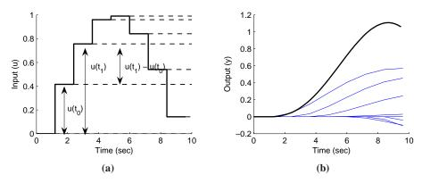
**Figure 5.2:** Response to piecewise constant inputs. A piecewise constant signal can be represented as a sum of step signals (a) and the resulting output is the sum of the individual outputs (b).
