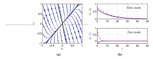
**Figure 5.5:** Illustration of the notion of modes for a second order system with real eigenvalues. The left figure (a) shows the phase plane and the modes corresponds to solutions that start on the eigenvectors (bold lines). The corresponding time functions are shown in (b).
