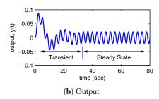
**Figure 5.8:** Transient versus steady state response. The left plot shows the input to a linear system and the right plot the corresponding output. The output signal initially undergoes a transient before settling into its steady state behavior.
