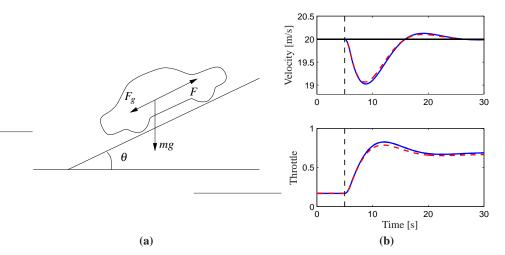
**Figure 5.14:** Simulated response of a vehicle with PI cruise control as it climbs a hill with a slope of  $4^{\circ}$ . The full lines is the simulation based on a nonlinear model and the dashed line shows the corresponding simulation using a linear model. The controller gains are  $k_p = 0.5$  and  $k_i = 0.1$ .
