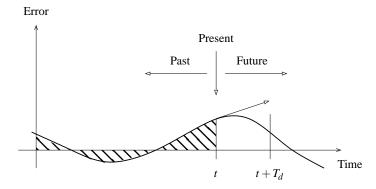
**Figure 1.17:** Action of a PID controller. At time *t*, the proportional term depends on the instantaneous value of the error. The integral portion of the feedback is based on the integral of the error up to time *t* (shaded portion). The derivative term provides an estimate of the growth or decay of the error over time by looking at the rate of change of the error.  $T_d$  represents the approximate amount of time in which the error is projected forward (see text).
