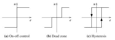
**Figure 1.16:** Input-output characteristics of on-off controllers. Each plot shows the input on the horizontal axis and the corresponding output on the vertical axis. Ideal on-off control is shown in (a), with modifications for a dead zone (b) or hysteresis (c). Note that for on-off control with hysteresis, the output depends on the value of past inputs.
