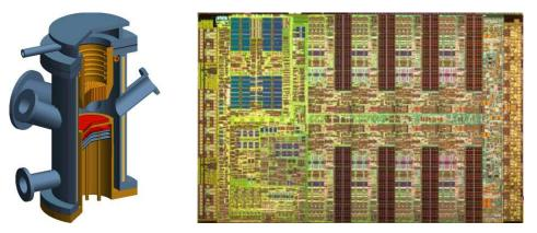
**Figure 1.7:** Materials processing. Modern materials are processed at carefully controlled conditions, using reactors such as the metal organic chemical vapor deposition (MOCVD) reactor shown on the left, which was for manufacturing superconducting thin films. Using lithography, chemical etching, vapor deposition and other techniques, complex devices can be built, such as the IBM cell processor shown on the right. Photographs courtesy of Caltech and IBM.
