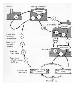
**Figure 1.11:** Supply chain dynamics (after Forrester [For61]). Products flow from the producer to the customer through distributors and retailers as indicated by the solid lines. The dashed lines show the upward flow of orders. The numbers in the circles represent the delays in the flow of information or materials. Multiple feedback loops are present as each agent tries to maintain the proper inventory levels.
