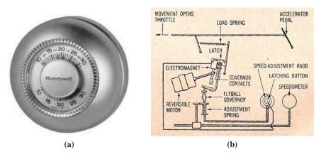
**Figure 1.4:** Early control devices. (a) Honeywell T86 thermostat, originally introduced in 1953. The thermostat controls whether a heater is turned on by comparing the current temperature in a room to a desired value that is set using a dial. (b) Chrysler cruise control system, introduced in the 1958 Chrysler Imperial [Row58]. A centrifugal governor is used to detect the speed of the vehicle and actuate the throttle. The reference speed is specified through an adjustment spring.
