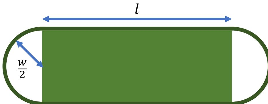
The basic idea is that the elastic cord loop goes through the top and bottom edge of the filter and forms two half-circles at its opposing ends. The filter is of width  $w$  and length  $l$  and must have a minimum area of  $300\text{cm}^2$  according to the standards. Moreover, they impose the following upper and lower bounds on the aspect ratio,
