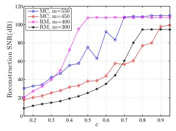
Fig. 3. Averaged SNR<sub>rec</sub> of the SRF algorithm as a function of c. Matrix dimensions are fixed to  $30\times30$  and r is set to 3. The parameter L and  $\epsilon$  are set to 8 and  $10^{-5}$ , respectively, to have small effect on this analysis. SNR's are averaged over 100 runs. 'MC' and 'RM' denote the matrix completion and affine rank minimization problems, respectively. For two MC problems, m is set to 450 and 550, and for two RM problems, m is set to 300 and 400.
