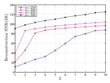
Fig. 2. Averaged  ${\rm SNR_{rec}}$  of the SRF algorithm in solving the ARM problem versus L. Matrix dimensions are fixed to  $30\times30$ , and r is set to 3. The parameter c and  $\epsilon$  are set to 0.9 and  $10^{-5}$ , respectively, to have small effect on this analysis. SNR's are averaged over 100 runs.
