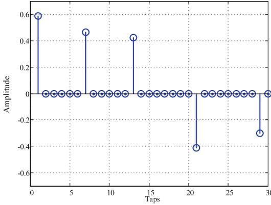
Fig. 1. Time domain discrete impulse response of a sparse channel
