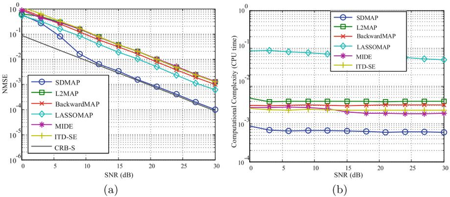
**Fig. 2.** Performance comparison. (a) NMSE versus SNR. (b) Computational complexity versus SNR
