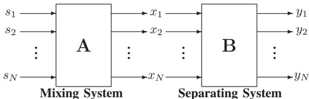
Figure 1: Mixing and separating systems in BSS.
