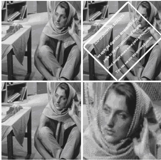
Fig. 4. The reconstruction of the masked image. (Top left) Original image. (Top right) The target regions are masked in white. (Bottom left) Region filling via the proposed inpainting algorithm. (Bottom right) The result of our algorithm around Barbara's eyes.
