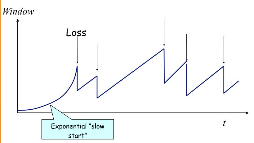
Why is it called slow-start? Because TCP originally had no congestion control mechanism. The source would just start by sending a whole receiver window's worth of data.
