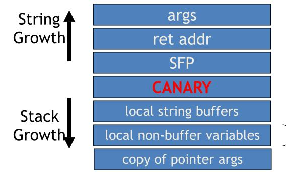
Protects pointer args and local pointers from a buffer overflow
