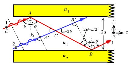
Two arbitrary waves 1 and 2 that are initially in phase must remain in after reflections. Otherwise the two will interfere destructively and ca other.
