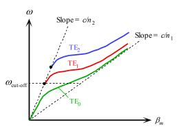
Schematic dispersion diagram,  $\omega$  vs.  $\beta$  for the slab waveguide for various TE<sub>m</sub> modes.  $\omega_{\text{cut-off}}$  corresponds to  $V = \pi/2$ . The group velocity  $v_g$  at any  $\omega$  is the slope of the  $\omega$  vs.  $\beta$  curve at that frequency.
