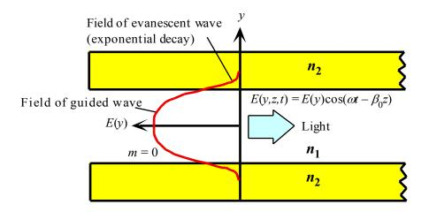
The electric field pattern of the lowest mode traveling wave along the guide. This mode has m = 0 and the lowest  $\theta$ . It is often referred to as the glazing incidence ray. It has the highest phase velocity along the guide
