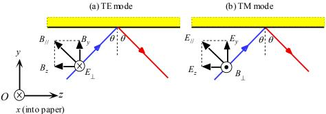
Possible modes can be classified in terms of (a) transelectric field (TE and (b) transmagnetic field (TM). Plane of incidence is the paper.
