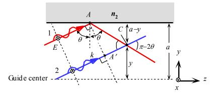
Interference of waves such as 1 and 2 leads to a standing wave pattern along the direction which propagates alongz.
