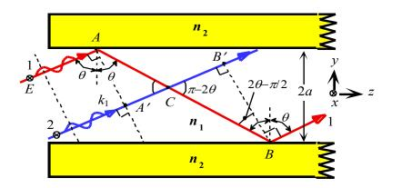
Two arbitrary waves 1 and 2 that are initially in phase must remain in after reflections. Otherwise the two will interfere destructively and ca other.
