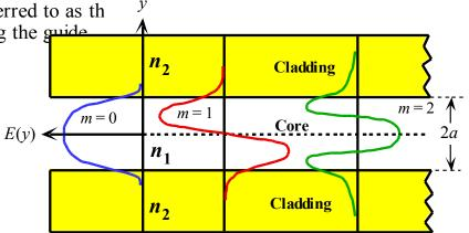
The electric field patterns of the first three modes (m = 0, 1, 2) traveling wave along the guide. Notice different extents of field penetration into the cladding.
