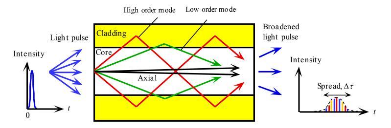
Schematic illustration of light propagation in a slab dielectric waveguide. Light pulse entering the waveguide breaks up into various modes which then propagate at differer group velocities down the guide. At the end of the guide, the modes combine to constitute the output light pulse which is broader than the input light pulse.
