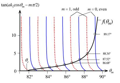
Modes in a planar dielectric waveguide can be determined by plotting the LHS and the RHS of eq. (11).
