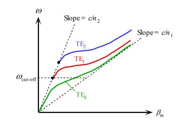
Schematic dispersion diagram,  $\omega$  vs.  $\beta$  for the slab waveguide for various TE<sub>m</sub> modes.  $\omega_{\text{cut-off}}$  corresponds to  $V = \pi/2$ . The group velocity  $v_g$  at any  $\omega$  is the slope of the  $\omega$  vs.  $\beta$  curve at that frequency.
