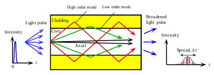
Schematic illustration of light propagation in a slab dielectric waveguide. Light pulse entering the waveguide breaks up into various modes which then propagate at differer group velocities down the guide. At the end of the guide, the modes combine to constitute the output light pulse which is broader than the input light pulse.
