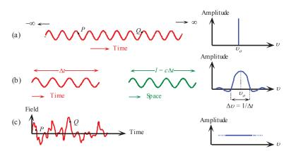
(a) A sine wave is perfectly coherent and contains a well-defined frequency  $v_o$ . (b) A finite wave train lasts for a duration  $\Delta t$  and has a length *l*. Its frequency spectrum extends over  $\Delta v = 1/\Delta t$ . It has a coherence time  $\Delta t$  and a coherence length *l*. (c) White light exhibits practically no coherence.
