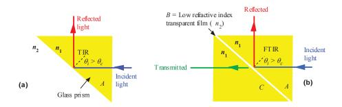
(a) A light incident at the long face of a glass prism suffers TIR; the prism deflects the light.
