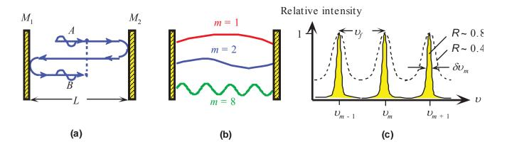
Schematic illustration of the Fabry-Perot optical cavity and its properties. (a) Reflected waves interfere. (b) Only standing EM waves, *modes*, of certain wavelengths are allowed in the cavity. (c) Intensity vs. frequency for various modes. R is mirror reflectance and lower R means higher loss from the cavity.
