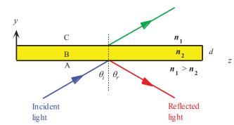
When medium B is thin (thickness d is small), the field penetrates to the BC interface and gives rise to an attenuated wave in medium C. The effect is the tunnelling of the incident beam in A through B to C.
