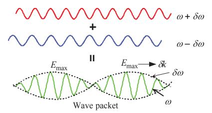
Two slightly different wavelength waves travelling in the same direction result in a wave packet that has an amplitude variation which travels at the group velocity.
