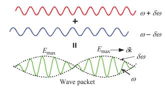
Two slightly different wavelength waves travelling in the same direction result in a wave packet that has an amplitude variation which travels at the group velocity.
