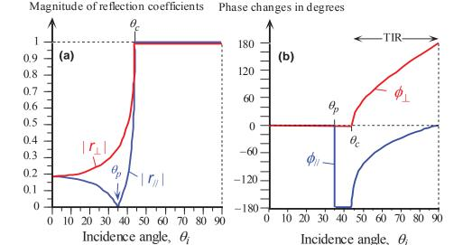
Internal reflection: (a) Magnitude of the reflection coefficients/ and  $r_{\perp}$  vs. angle of incidence  $\theta_i$  for  $n_1 = 1.44$  and  $n_2 = 1.00$ . The critical angle i 44°. (b) The corresponding phase changes  $\phi_{//}$  and  $\phi_{\perp}$  vs. incidence angle. © 1999 SO. Kasap, *Optoelectronics* (Prentice Hall)
