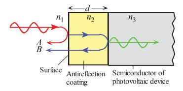
Illustration of how an antireflection coating reduces the reflected light intensity
