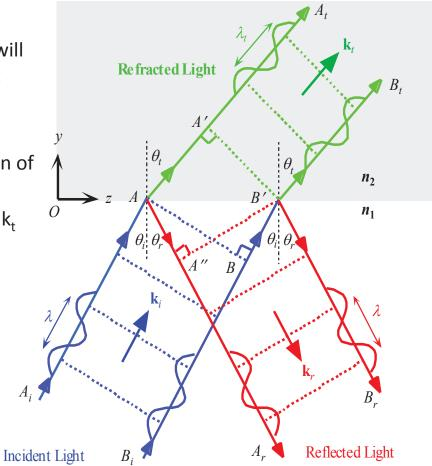
A light wave travelling in a medium with a greater refractive index  $(n_1 > n_2)$  suffers reflection and refraction at the boundary.
