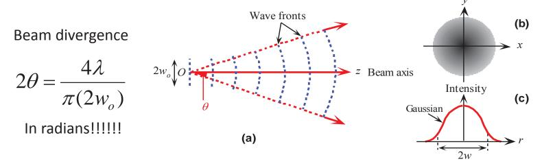
(a) Wavefronts of a Gaussian light beam. (b) Light intensity across beam cross section. (c) Light irradiance (intensity) vs. radial distancer from beam axis (z).
