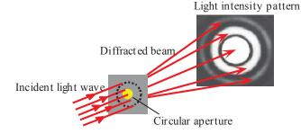
A light beam incident on a small circular aperture becomes diffracted and its light intensity pattern after passing through the aperture is a diffraction pattern with circular bright rings (called Airy rings). If the screen is far away from the aperture, this would be a Fraunhofer diffraction pattern.
