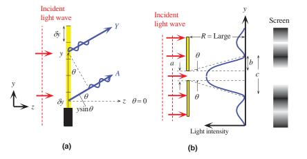
• The single slit diffraction equation yields an intensity  $(1)^{2}$
