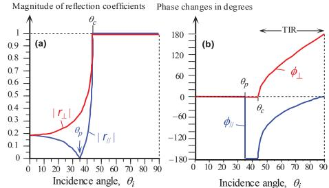
Internal reflection: (a) Magnitude of the reflection coefficients/ and  $r_{\perp}$  vs. angle of incidence  $\theta_i$  for  $n_1 = 1.44$  and  $n_2 = 1.00$ . The critical angle i 44°. (b) The corresponding phase changes  $\phi_{l/}$  and  $\phi_{\perp}$  vs. incidence angle © 1999 SO. Kasap, *Optoelectronics* (Prentice Hall) 31
