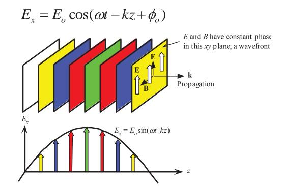
A plane EM wave travelling along z, has the same  $E_x$  (or  $B_y$ ) at any point in a given xy plane. All electric field vectors in a given xy plane are therefore in phase. The xy planes are of infinite extent in the x and y directions.
