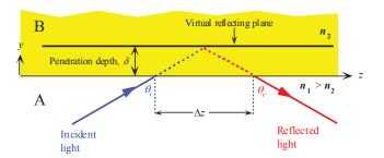
The reflected light beam in total internal reflection appears to have been laterally shifted by an amount  $\Delta z$  at the interface.
