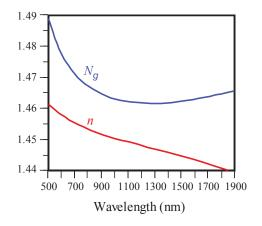
Refractive index *n* and the group index  $N_g$  of pure SiO<sub>2</sub> (silica) glass as a function of wavelength. © 1999 S.O. Kasap, *Optoelectronics* (Prentice Hall)
