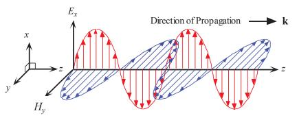
An electromagnetic wave is a travelling wave which has time varying electric and magnetic fields which are perpendicular to each other and the direction of propagation,*z*.
