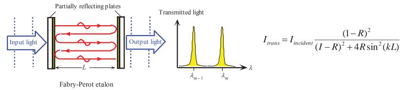
Transmitted light through a Fabry-Perot optical cavity.
