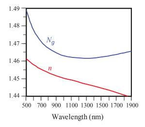
Refractive index n and the group index  $N_g$  of pure SiO<sub>2</sub> (silica) glass as a function of wavelength.
