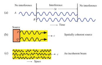
(a) Two waves can only interfere over the time interval $\lambda t$ . (b) Spatial coherence involves comparing the coherence of waves emitted from different locations on the source. (c) An incoherent beam.
