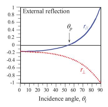
The reflection coefficients  $r_{//}$  and  $r_{\perp}$  vs. angle of incidence  $\theta_i$  for  $n_1 = 1.00$  and  $n_2 = 1.44$ .
