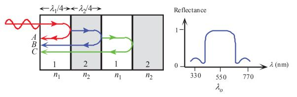
Schematic illustration of the principle of the dielectric mirror with many low and high refractive index layers and its reflectance.
