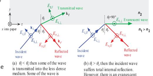
Light wave travelling in a more dense medium strikes a less dense medium. The plane of incidence is the plane of the paper and is perpendicular to the flat interface between the two media. The electric field is normal to the direction of propagation. It can be resolved into perpendicular ( $\bot$ ) and parallel (//) components 28
