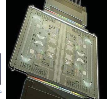
240 Optical components on a chip -Infinera Wavelength Multiplexer2007
