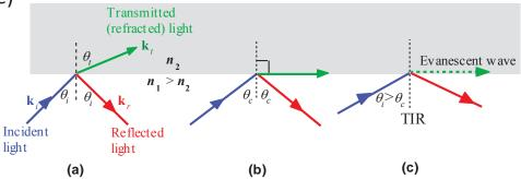
Light wave travelling in a more dense medium strikes a less dense medium. Depending on the incidence angle with respect to  $\theta_c$ , which is determined by the ratio of the refractive indices, the wave may be transmitted (refracted) or reflected. (a)  $\theta_i < \theta_c$  (b)  $\theta_i = \theta_c$  (c)  $\theta_i > \theta_c$  and total internal reflection (TIR).
