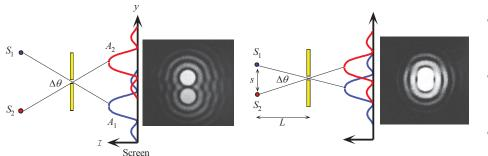
Resolution of imaging systems is limited by diffraction effects. As points  $S_1$  and  $S_2$  get closer, eventually the Airy disks overlap so much that the resolution is lost.
