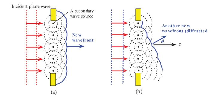
(a) <u>Huygens-Fresnel principles</u> states that each point in the aperture becomes a source of secondary waves (spherical waves). The spherical wavefronts are separated by  $\lambda$ . The new wavefront is the envelope of the all these spherical wavefronts. (b) Another possible wavefront occurs at an angle  $\theta$  to the *z*-direction which is a diffracted wave.
