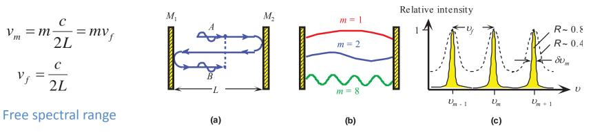
$$\Delta v_m = v_{m+1} - v_m = v_m$$
