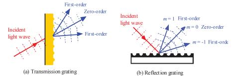
(a) Ruled periodic parallel scratches on a glass serve as a transmission grating. (b) A reflection grating. An incident light beamresults in various "diffracted" beams. The zero-order diffracted beam is the normal reflected beam with an angle of reflection equal to the angle of incidence.
