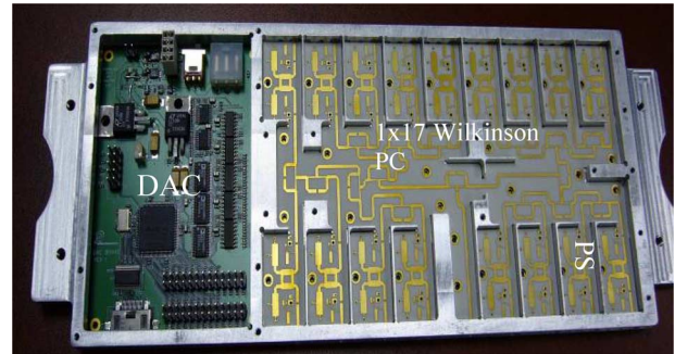
Fig. 7. Phase shifter power combiner box and DAC board.
