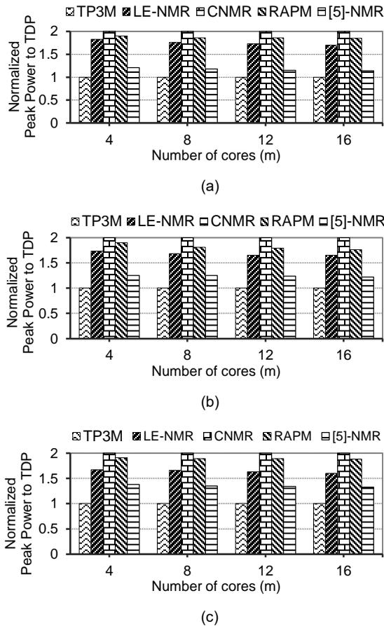
Fig. 5. Normalized peak power to the chip TDP in the worst-case scenario. a) Low parallelism degree, b) Medium parallelism degree, c) High parallelism degree.
