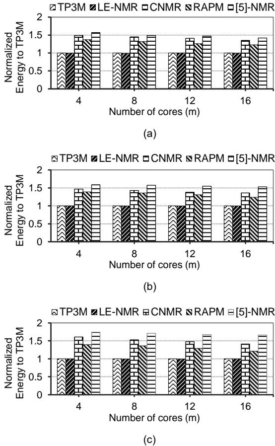
Fig. 7. Normalized energy consumption to TP3M in the worst-case scenario. a) Low parallelism degree, b) Medium parallelism degree, c) High parallelism degree.
