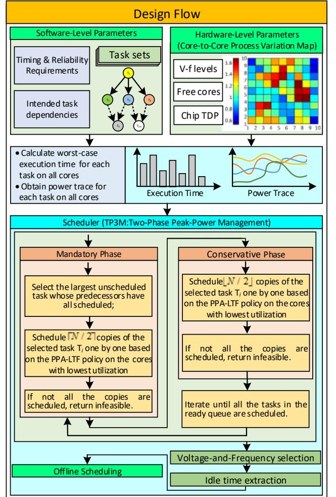
Fig. 2. The operational flow of our TP3M system.
