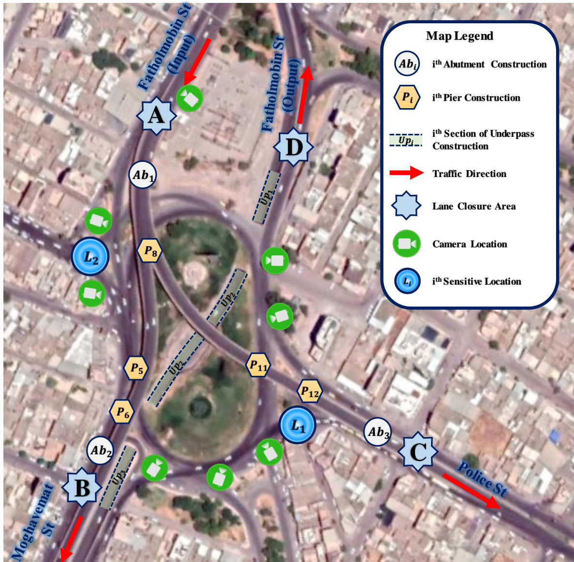
Figure 2. Project plan view representing traffic directions, grade separation construction elements, and sensitive locations.
