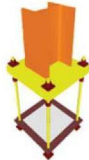
LOD 400 – Construction details, including connection information
