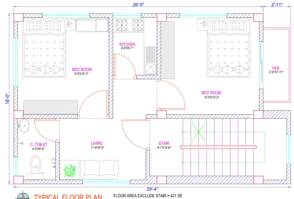
TYPICAL FLOOR PLAN SCALE: 1/3"=1'-0"
