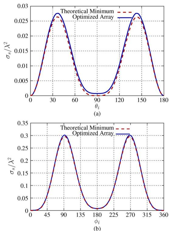
Fig. 4. Normalized total scattering cross section versus the angle of incidence. Solid lines represent the total scattering cross section obtained from method of moments (MoM) analysis, and dashed lines show the lower bound from (17). (a) E-plane or  $xoz$ -plane. (b) H-plane or  $xoy$ -plane.
