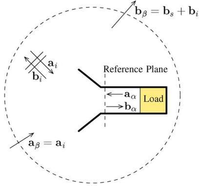
Fig. 1. Receiving antenna under illumination of a plane wave.
