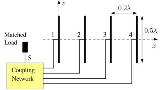
Fig. 2. Four-element equispaced half-wave dipole array. The incident plane wave is linearly polarized along the  $z$ -axis and is traveling along the  $x$ -axis.
