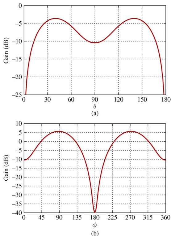
Fig. 3. Antenna gain after minimization of the scattered power. (a) E-plane. (b) H-plane.
