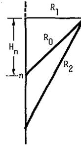
Fig. 2. Geometry for evaluation of  $Z_{mn}$ .
