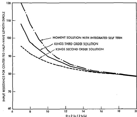
Fig. 8. Input resistance of half-wavelength dipoles for varying  $h/a$ .
