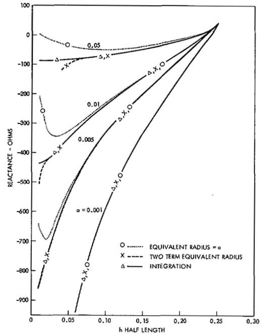
Fig. 4. Reactance of dipole versus half-length comparing results of integration and two term equivalent radius.
