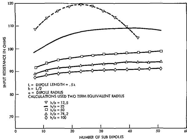
Fig. 7. Input resistance of half-wavelength dipoles versus number of subsections.
