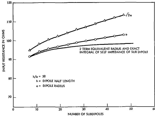
Fig. 6. Input resistance of half-wavelength dipole with  $h/a = 50$ .
