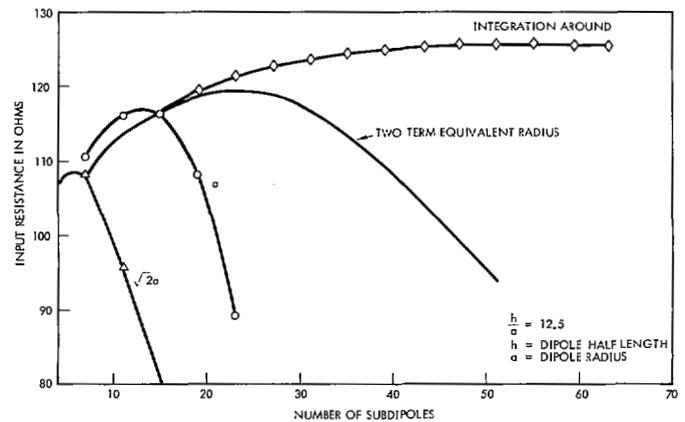
Fig. 5. Input resistance of half-wavelength dipole with  $h/a = 12.5$ .
