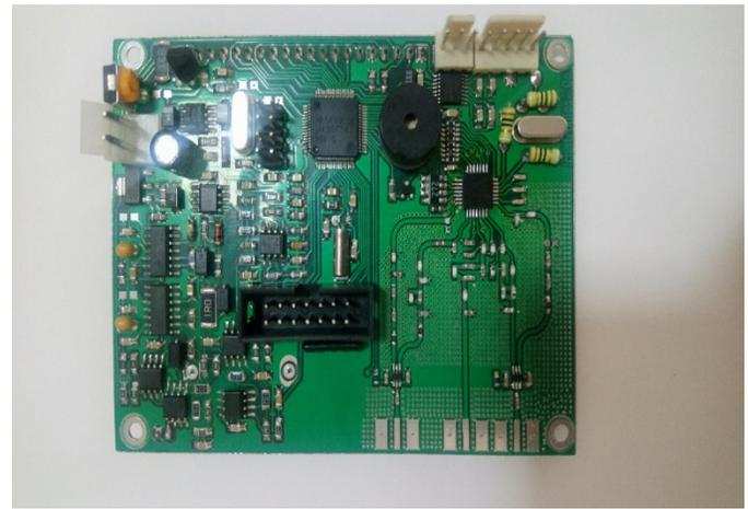
Fig. 10: The implemented node consists of a power measurement unit, a power supply, a processor, LoRa transceiver, and an RS232 communication port.
