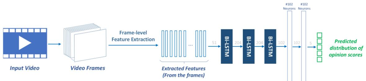
**Figure 1.** Overview of the proposed method: after the feature extraction stage, a recurrent neural network transforms the features into a distribution of quality scores at its output layer. The gray numbers indicate the output dimension of each layer. The inputs to the Bi-LSTM units are sequences of vectors each with the specified dimensions
