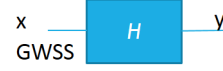
Fig. 2. Passing a GWSS process through a graph filter, results in a GWSS process.
