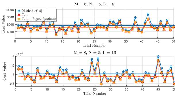
Fig. 3: Comparison of the obtained cost function values using the waveform design method of [2], P. 1, and P. 1 + signal synthesis. Average values have been shown by straight lines.
