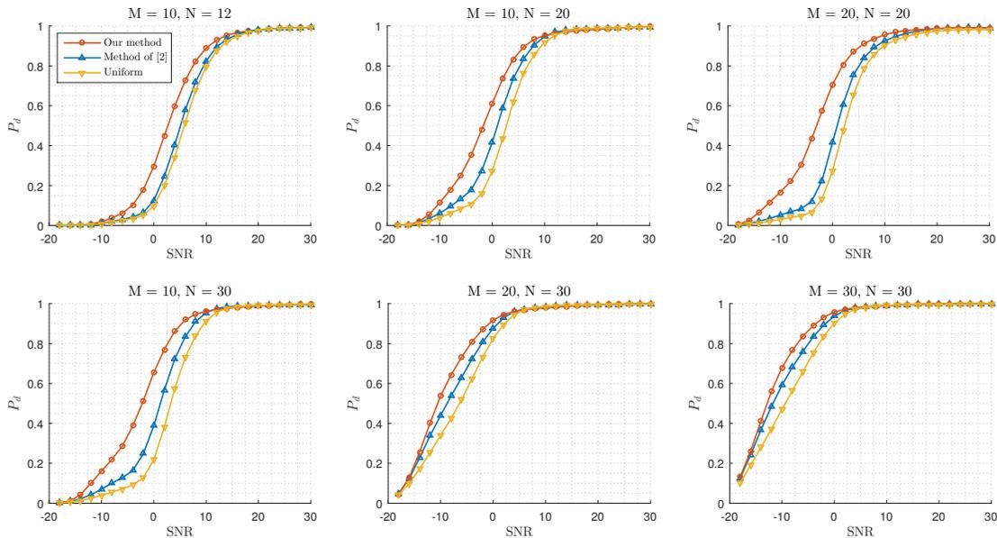
Fig. 2:  $P_d$  vs. SNR for different power allocation methods,  $P_{fa} = 10^{-4}$ ,  $L = 32$ .
