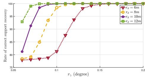
Fig. 1: Rate of correct support estimation vs. angular resolution ( $r_\gamma$ ).
