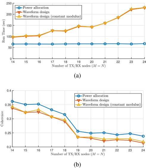
Fig. 6: Comparison of power allocation and waveform design for (a) run time and (b) coherence measure.
