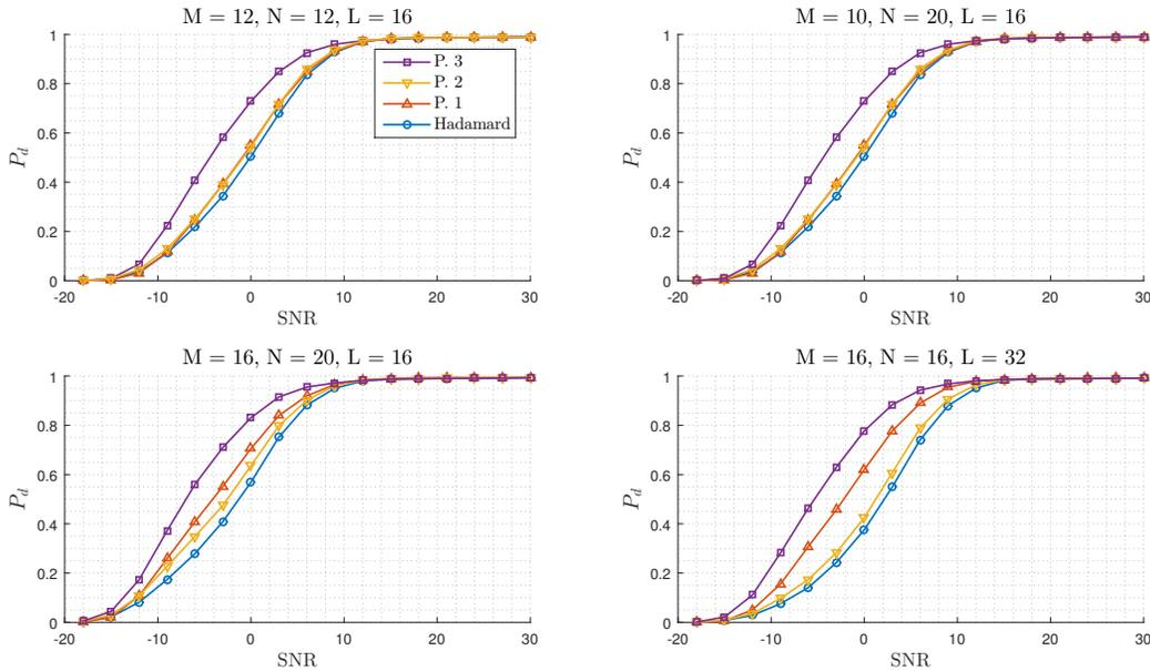
Fig. 5:  $P_d$  vs SNR for different waveform design methods,  $P_{fa} = 10^{-4}$ .
