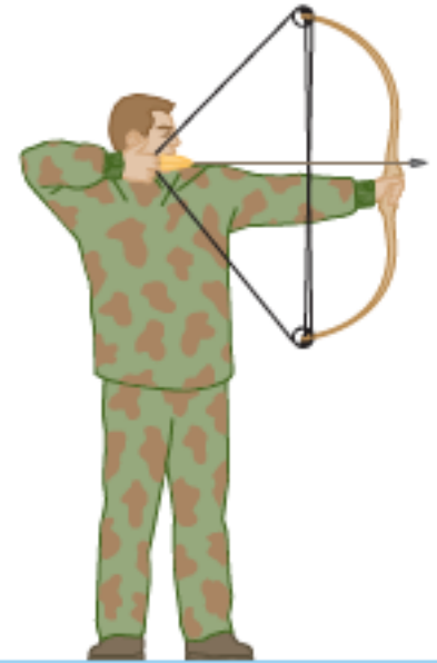
Figure 9.2 (Example 9.1) An archer fires an arrow horizontally to the right. Because he is standing on frictionless ice, he will begin to slide to the left across the ice.
