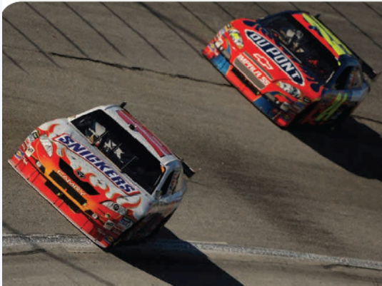
Kyle Busch, driver of the #18 Snickers Toyota, leads Jeff Gordon, driver of the #24 Dupont Chevrolet, during the NASCAR Sprint Cup Series Kobalt Tools 500 at the Atlanta Motor Speedway on March 9, 2008 in Hampton, Georgia. The cars travel on a banked roadway to help them undergo circular motion on the turns. (Chris Graythen/Getty Images for NASCAR)
