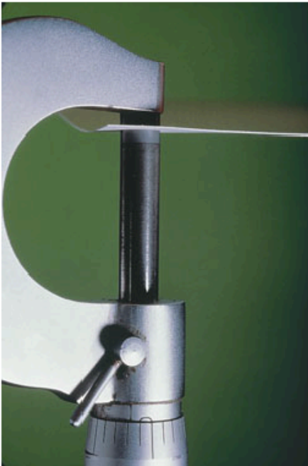
FIGURE 1–11 Example 1–7. Micrometer used for measuring small thicknesses.
