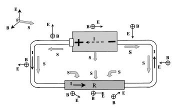
Fig. 4. The electric and magnetic fields, **E** and **B**, and Poynting vector **S** along the closed dc circuit. The case of ideal wires, homogeneous resistor R, and ideal source with no internal resistance is considered.
