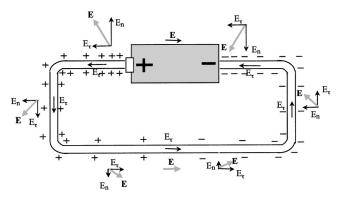
Fig. 2. The rotation of the electric field  $\mathbf{E}$  ( $E_n$ ,  $E_\tau$ ) outside and along the closed dc circuit. Inside the wire the electrical field is collinear with the wire ( $E_\tau$ ). The case of a homogeneous wire and an ideal source with no internal resistance is considered.
