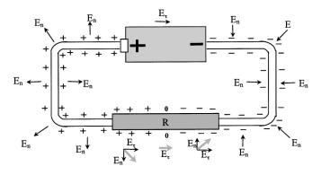
Fig. 3. The electric field  $\mathbf{E}$  along and outside the closed dc circuit. The case of ideal wires, homogeneous resistor R, and ideal source with no internal resistance is considered.
