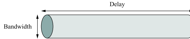
Figure 1.21 Network as a pipe.
